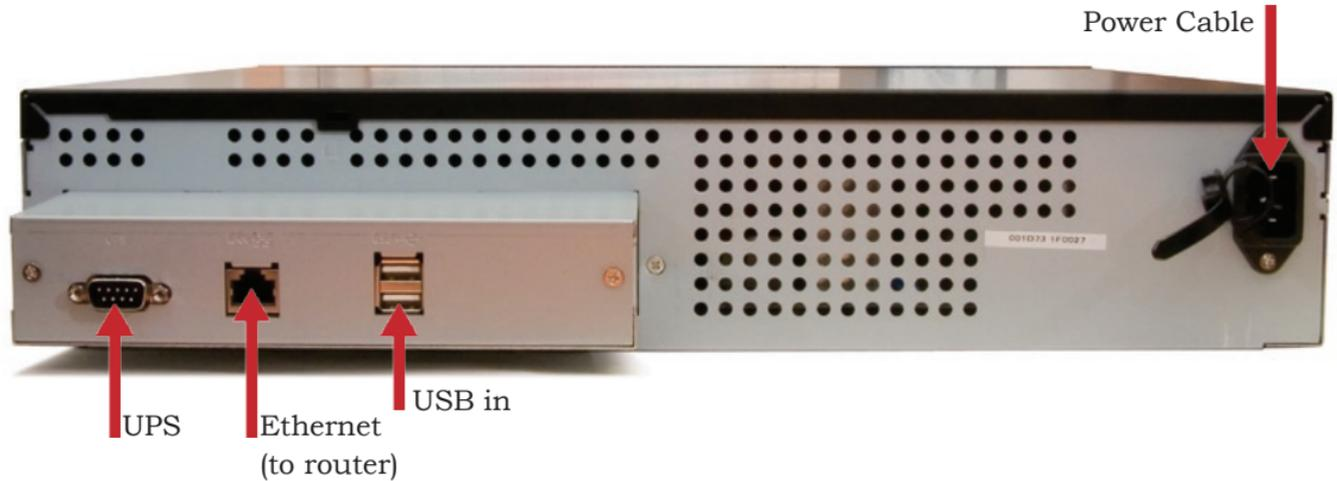
Begin by connecting your TeraStation's power and Ethernet cables. For best results, the Ethernet cable should be connected to a router, hub, or switch on your network. Turn the TeraStation on by pushing the power button on the front panel. It will take about a minute to boot.
