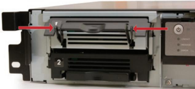
Squeeze the tabs gently and swing the tray latch upward.
